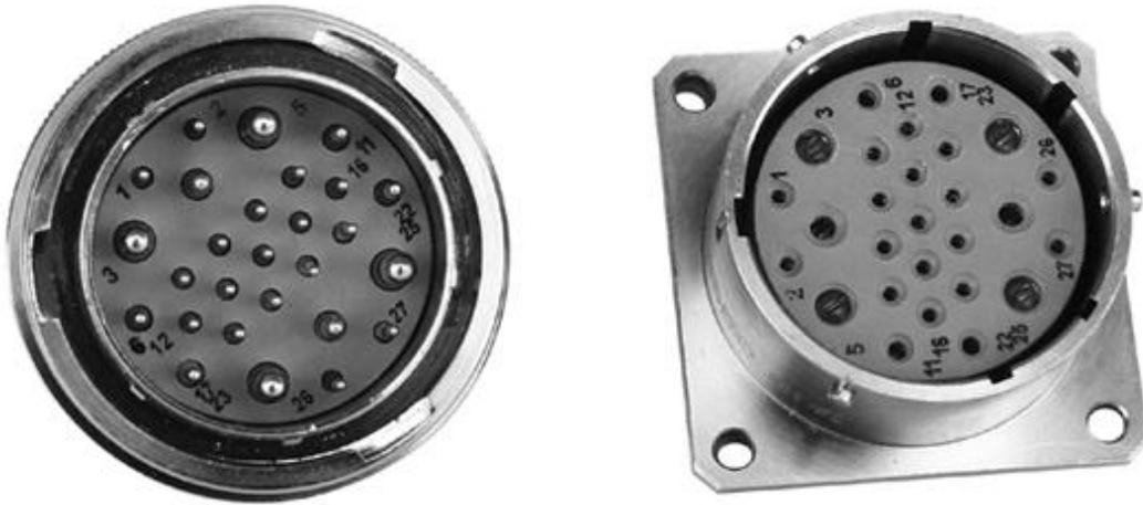
Conform to Chinese military connector standard GJB2889, CXCH-01 series is extended from XC series, designed as bayonet coupling, solder or crimp springtac contact. The difference from XC series is thicker shell and stronger anti-vibration.
